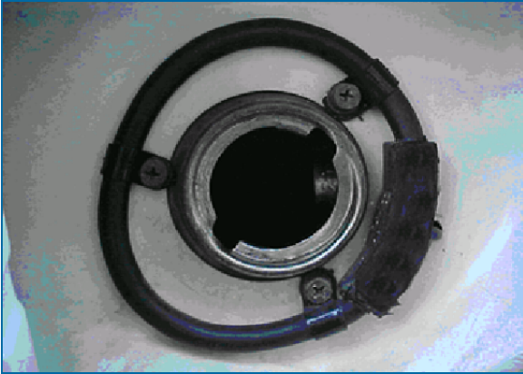
Figure 3-1 Tag with P-Clips Installed
