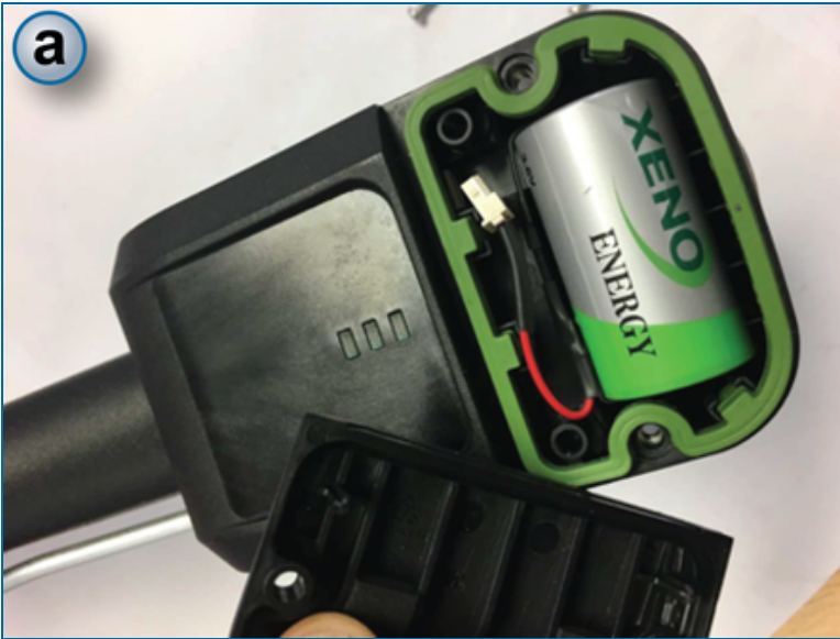
a. Remove the battery cover screws and open the battery compartment.
