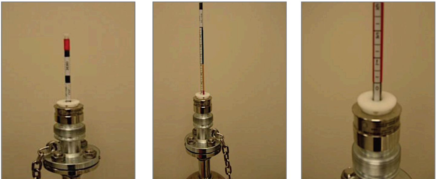
Figure 2-1 Gage Rod Moves Upwards to Provide Level Measurement Reading
